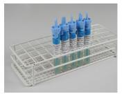
7 Place the EliA Stool Extraction Kit *plus* into a universal sample rack and allow it to stand (extract) for a minimum of 10 minutes before measurement. For all subsequent steps, handle tube in a gentle manner to avoid disturbing the sediment.
