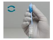
8 Hold the device upright and remove the sampling probe and the dark blue adapter together by turning the adapter in a counter-clockwise direction. Dispose of sampling probe and adapter, treating both as biohazardous material.
