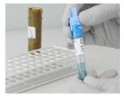
**4** Carefully insert the light blue sampling probe through the dark blue adapter into the tube.
