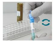
**5** Lock the tube firmly by turning the probe grip of the sampling probe in a clockwise direction.
