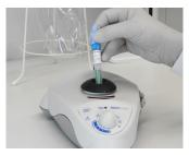
6 Hold the device on a vortex mixer which is set at full speed. After the stool sample has been released from the grooves, ensure a minimum vortex time of 20 seconds.
