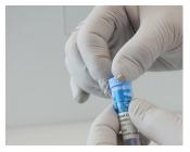
**1** Remove the light blue sampling probe by turning the light blue probe grip in a counter-clockwise direction.
